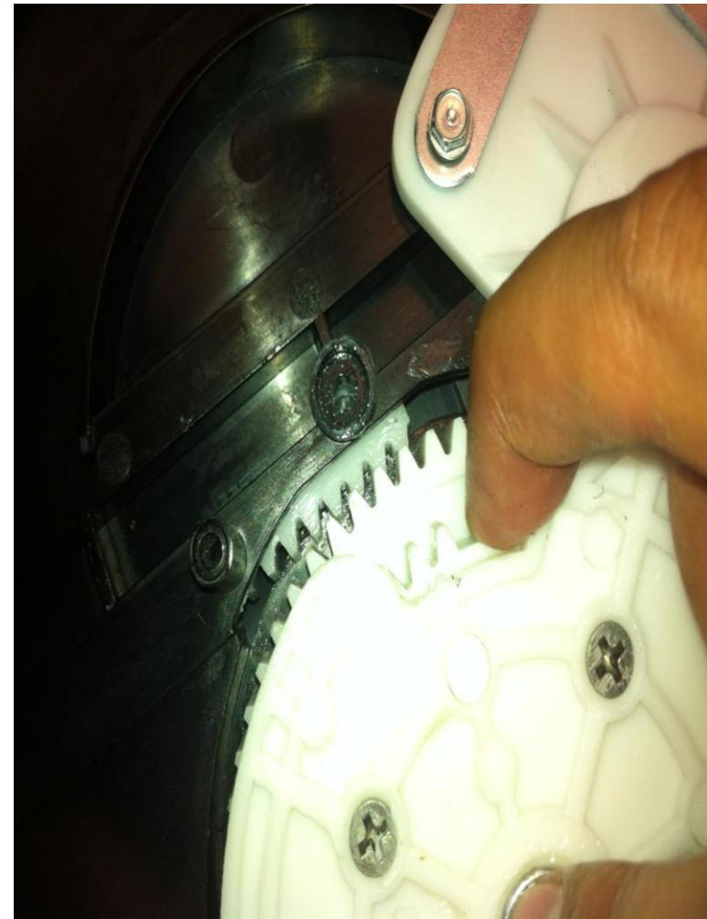
ONCE GEAR/CAM IS ALIGNED AND LOCKED IN PLACE, PLACE CAM LINK NEXT TO GEAR AND ALIGN TEETH SO THE TOOTH ON THE GEAR LINK IS AT THE TOP OF THE ENGAGEMENT.
